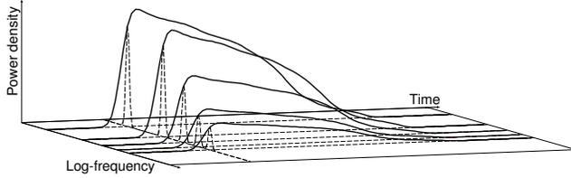
Fig. 1. Profile of a HTC source model  $q_k(x, t; \Theta)$
